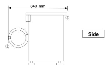
(When The Door Vertically Open ) The distance between door① and the rear side② is 760mm
